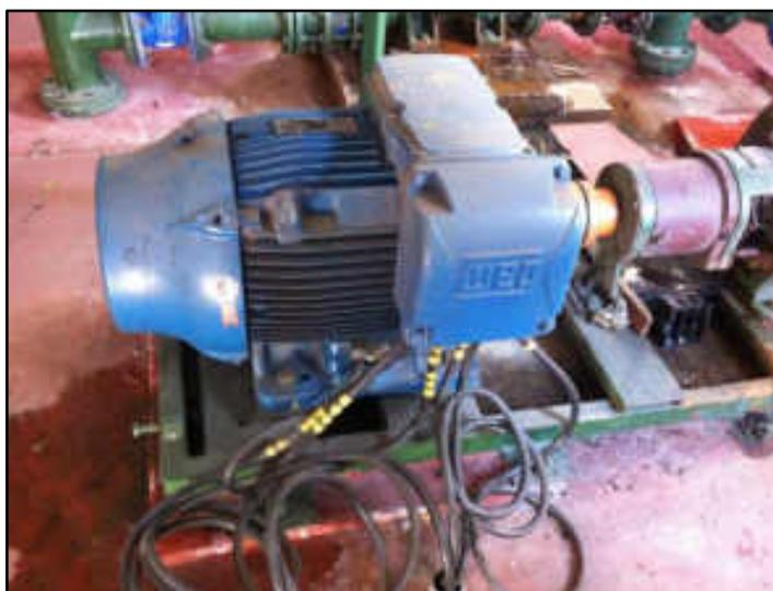
6.1 MOTOR DE INDUÇÃO WEG W 22 PLUS 3560 RPM HP 75 100 CV 60 HZ 220 380 440 V
